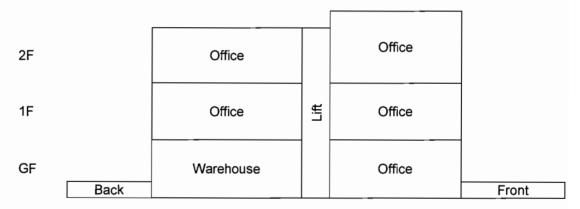
Type B comprises a full office-like building inclusive of a portion for production or warehousing on the ground floor. Both the second floor and third floor comprises office or production space. This design is ideal for various business needs and can be used as an administrative office, showroom, storage space, studio and production house, display space and others.
