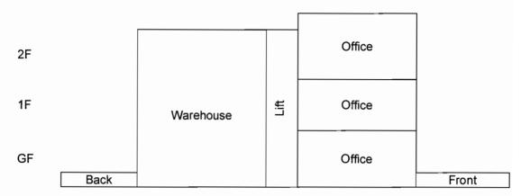
Type A comprises an office or production space at the front portion and double-volume factory or warehouse at the rear given its high ceiling warehouse layout. This design provides flexibility as it can meet the needs of various minor industrial processes and production purposes. Further, it can also be converted into research laboratories, warehouses and storage space for various materials.
